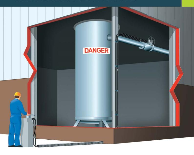
The cable system can be passed through walls, bulkheads, floors and any other obstacles to reach the valve.
